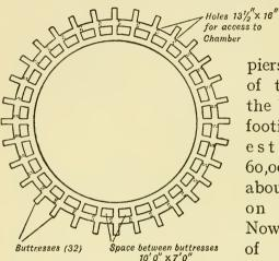
FIG. 20.—HORIZONTAL SECTION AT X-Y OF WALLS CARRYING DOME (see Fig. 18) SHOWING BUTTRESSES AND CHAMBERS AT LEVEL OF WHISPERING GALLERY.
